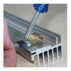
Practical tool for assembly clips of Alutronic
